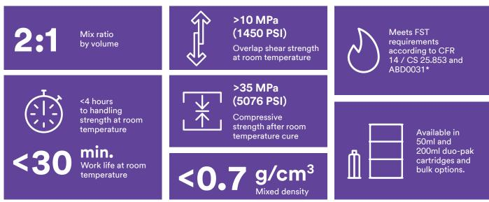
\* Tested in accordance with §25.853 (a), Appendix F, Part I (a) (1) (ii), 12-second vertical burn per FAA Policy Statement PS-ANM-25.853-01-R2, Reference 23, Option 1 (in a stand-alone mode, cured test plaque of nominal size: 0.25" x 3" x 12"); §25.853 (d), Appendix F, Part V, smoke density; and AITM 3.0005, smoke toxicity. Installation approval is the responsibility of the design approval holder or the aircraft owner/operator.
