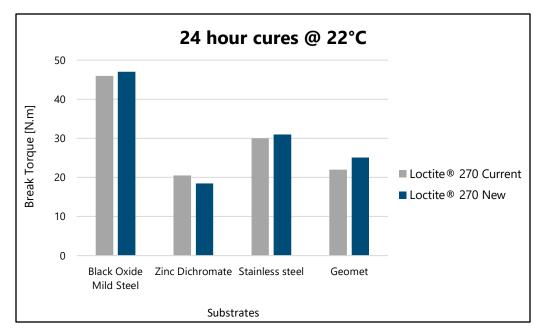
**Conclusion:** Overall comparable strength observed for Loctite® 270 Current and Loctite® 270 New.
