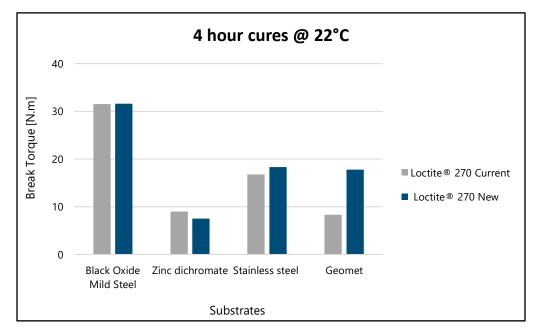
**Conclusion:** Consistent cure performance is observed for Loctite® 270 Current and Loctite® 270 New on all substrates tested.
