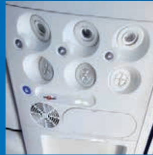
Ceiling panels/ducts/ passenger service units (PSU)
