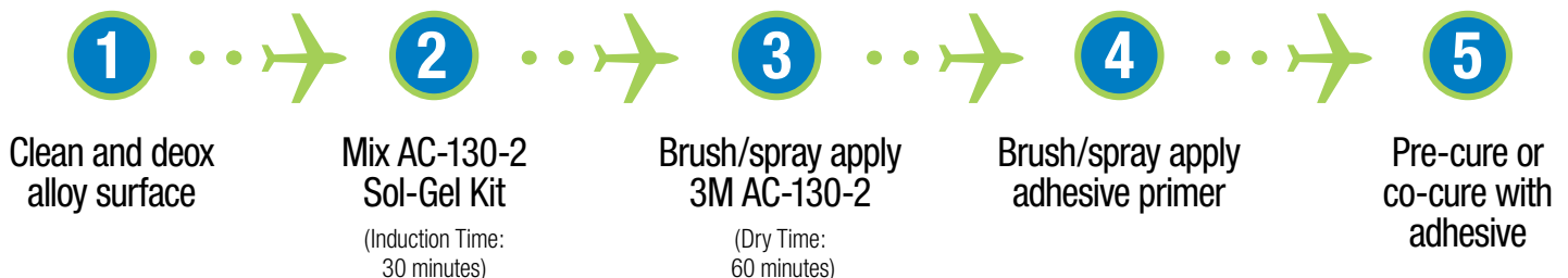
Figure 2. Surface treatment process using 3M AC-130-2
